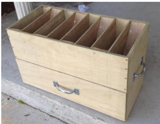
*Figure 7.* Ply wood manufactured riffle box
