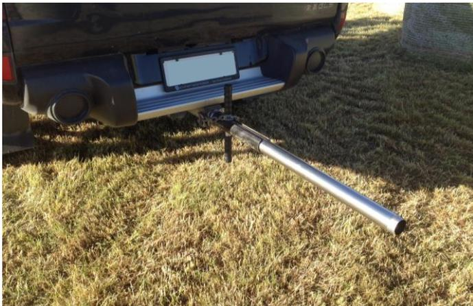
*Figure 3.* Corer and bracket fixed to a 4WD. Design appendix V
